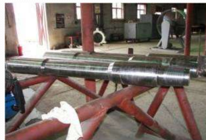
SOME OF MSL'S FINISHED PRODUCTS- MACHINING 6 5/8" DIA PIN BY HT 55 BOX
